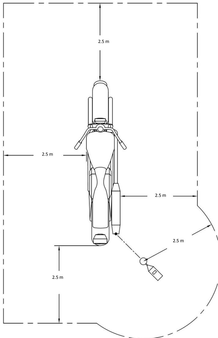
**Figure A.2: Position of the microphone in relation to the exhaust pipe.**
