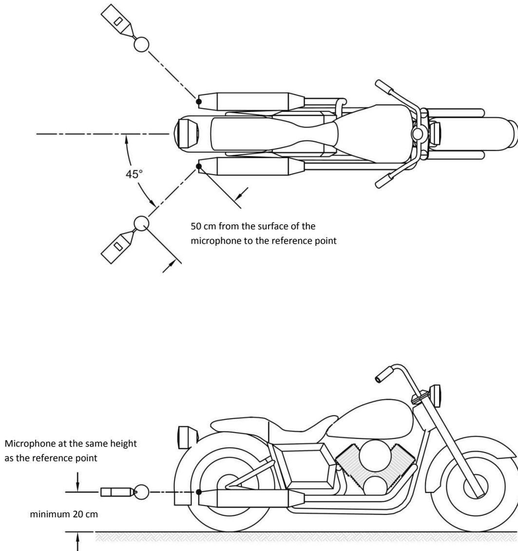
**Figure A.3: Exhaust pipes to choose when there are several pipes on the same side.**
