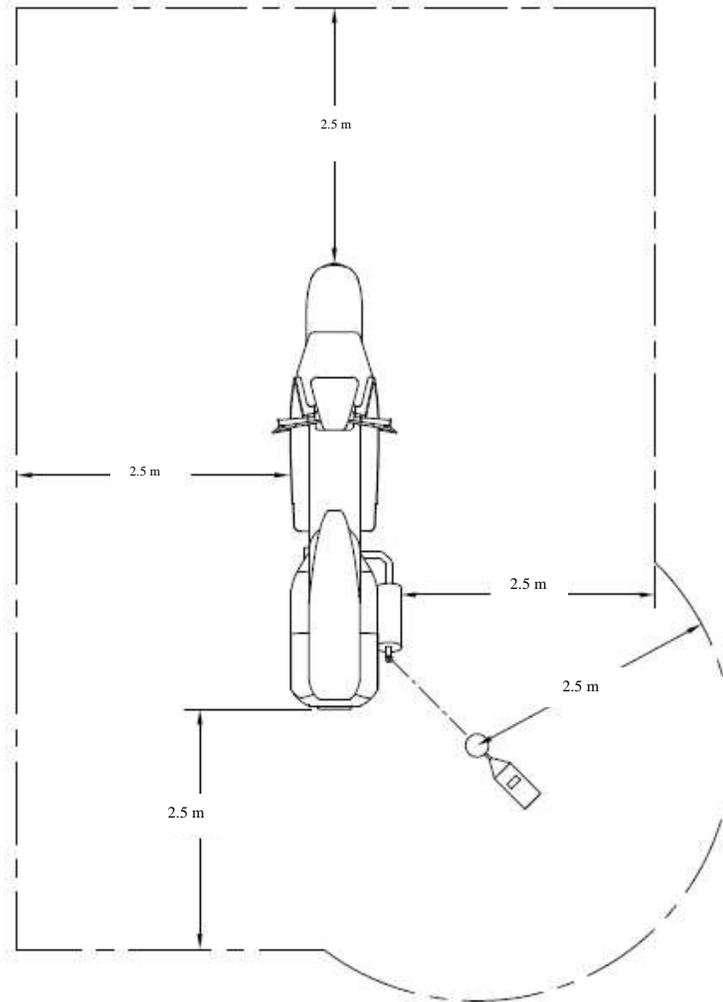
**Figure A.2: Position of the microphone in relation to the exhaust pipe**
